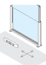
For proper function of OPEN AIR units, the installation must be only on concrete or tiled floors.
