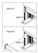
**Step 4** We take the motor out in (2) moves. We slide it upwards from both sides, and we take it out through the special cutting onto profile 2200-1111.
